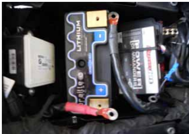
Installing the new Braille Lithium Battery
