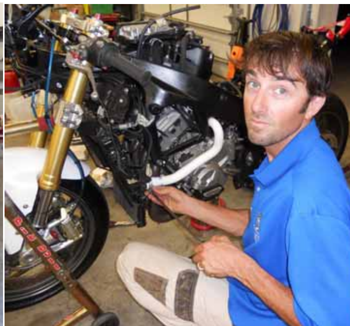
Shane Applegate installs new Samco hoses
